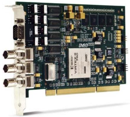
“It supports 1080i, 1080p and 720p resolutions with 8 channels of AES/EBU digital audio. With simultaneous standard definition down-conversion for viewing HD content on an SD-SDI broadcast monitor, the HD-SDI Master is well suited for video
