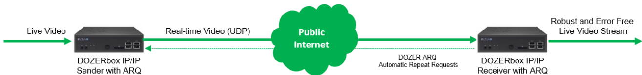
Figure 1: DOZER ARQ Pair Enables Error-free Live Video over the Internet
