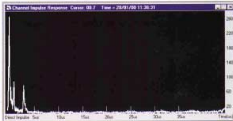
GRAPH 2 Plotting of Impulse Response showing signal and echoes, using pc package. Here, two echoes can clearly be seen in the time domain.
